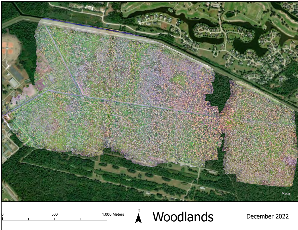
Figure 7. December 2022: Woodlands Preserve drone-derived orthomosaic of VARI (top) and visible (below) imagery. VARI scale is dimensionless; orange = less vegetation/sparse canopy, green = more vegetation/contiguous canopy.
